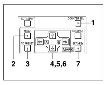
1 Press the COUNTER SEL button to light the time data type indicator "TC" or "U-BIT."
